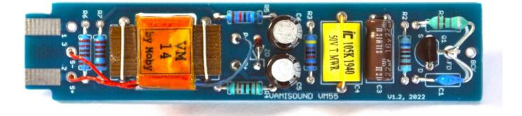
Notice the two white dots (or black on some pieces) on the transformer near the bottom edge of the circuit board. They mark the beginning of the transformer windings and will help you solder the wires into the correct holes.
