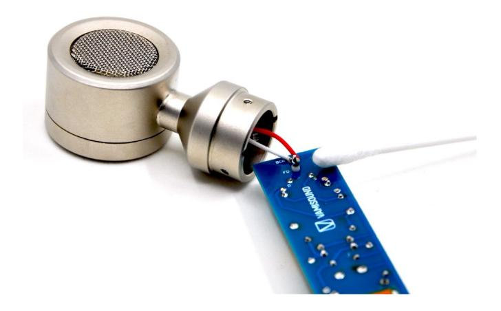
At this stage you can carefully connect the microphone to the preamp and measure the voltage on the XLR pins and on the different points of the circuit (on zener diode, on drain and source of FET).
