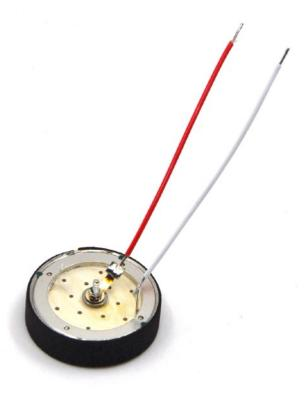
Take the microphone head and insert the rear grille, then the grey spacer ring with the circular cutout as you see in the picture. Finally insert the capsule, put the front grille on top of it and then screw everything together.
