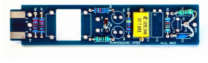
In next sequence install electrolytic capacitor C3. Also pair of caps C5 and C6. Place fet transistor Q1 in place and solder its pin to the teflon pin.
