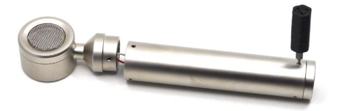
Now comes probably the most tricky part of the whole construction. Be patient and do it very carefully and slowly. You have to fit the circuit board into the two rails in the head section of the microphone and then fit the whole microphone tube.
