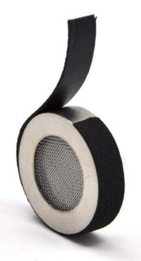
Then insert the taped capsule into the microphone head as shown. It's just to test that capsule sitting there. Don't put it all the way in yet.
