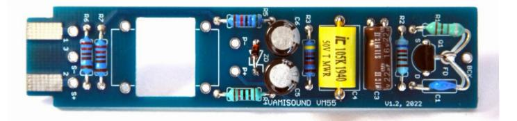
Install output transformer VM14. Attach the transformer using the two cutted legs from the resistors to the board. Make sure the transformer does not wobble on the board.
