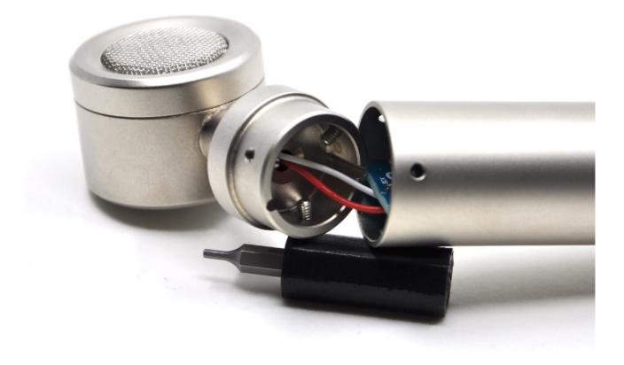
Before you close the microphone completely make sure that the circuit board fits snugly into the two cutouts (rails) in the head section of mic and that the microphone cables are not pinched anywhere.
