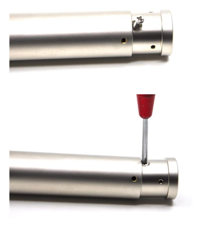
Carefully unscrew (= counterclockwise) the three hexagonal screws from the bottom out into the microphone tube. Again, be careful not to unscrew these screws all the way out of the tube. Screw them out only about to the edge of the microphone tube so that they do not protrude.
