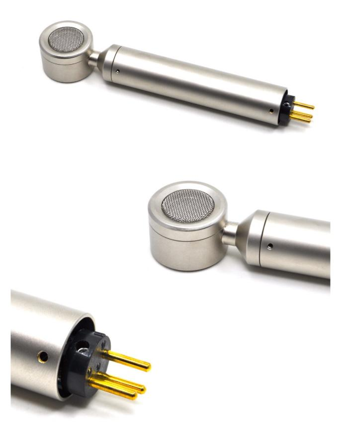
Now screw the bottom of the microphone and the XLR insert together.
