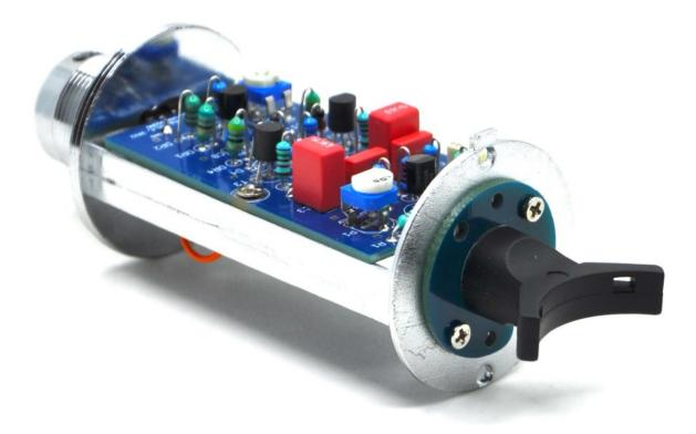
Now it's time to attach your favorite capsule to the holder. As stated earlier the Schoeps LDC is a frequency flat circuit very suitable for capsules like C12, K47 or M7 that do not need frequency correction.
