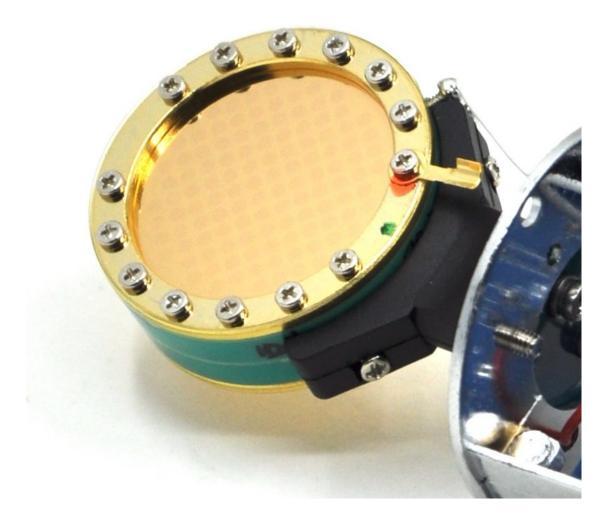
Solder the cable from the front diaphragm to the teflon pin on the underside of the board.
