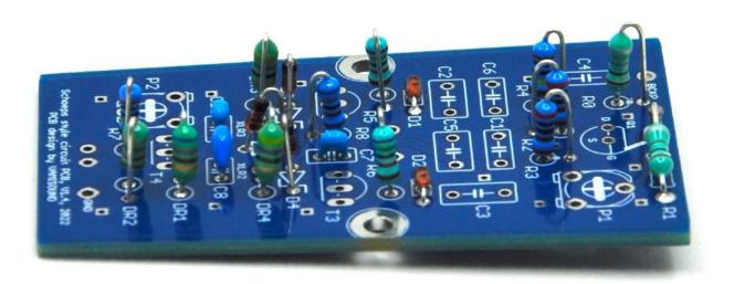
Film capacitors always light up the whole board :-) Don't install C5 now. You can use this with a very bright capsules. C5 forms LPF. Experiment with values around 22nF if necessary.
