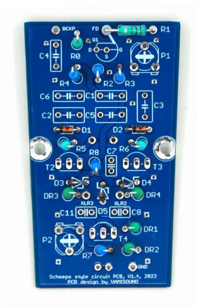
Continue with ceramic capacitors C7, C8 and C11.
