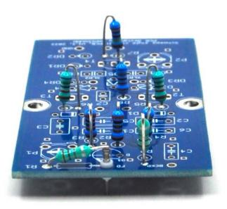
Continue by soldering diodes D1 and D2.
