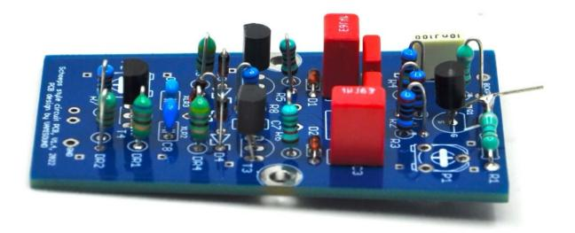
Solder the two trimmer resistors into their place.
