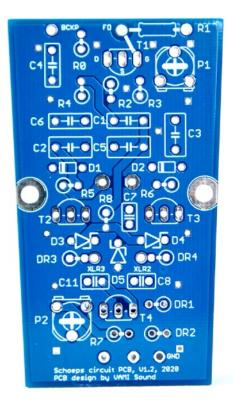
Solder all resistors according to the BOM first and install teflon pin by hole on the board marked as "FD". Note that R1 is soldered with one leg to this teflon pin – in the air.
