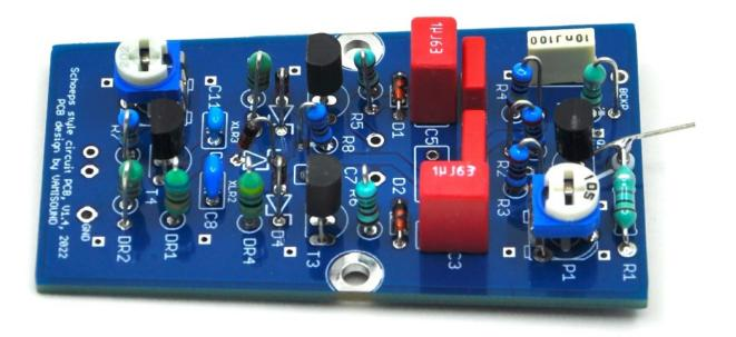
Now it's time to carefully clean the bottom side of the printed circuit board. Isopropyl alcohol and a toothbrush is your good helper.
