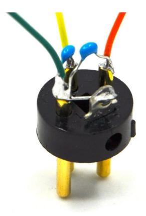
Screw the prepared XLR connector into the microphone chassis.
