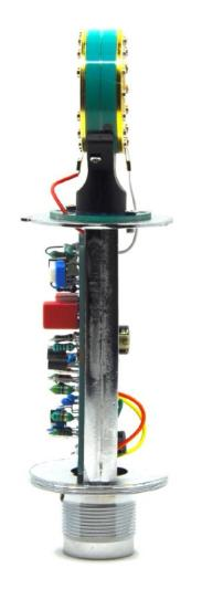
Solder the cable from the backplate to the pad marked BCKP on the circuit board.
