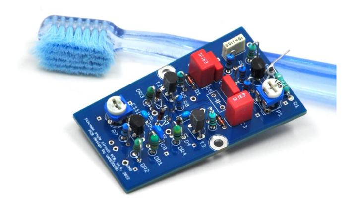
After cleaning the board, solder two electrolytic capacitors from the bottom side of the board.
