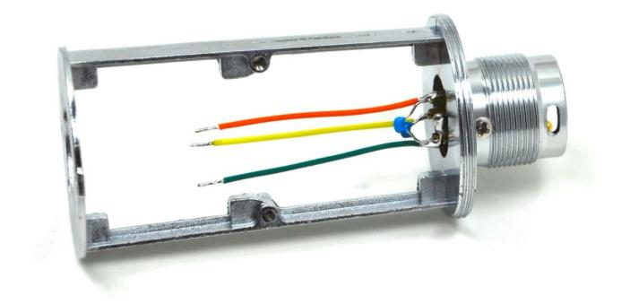
Screw the microphone board to the chassis and solder the three cables to the appropriate pads on the board.
