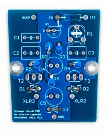
Install the teflon pin and the remaining R1 that feeds into it as if in air.
