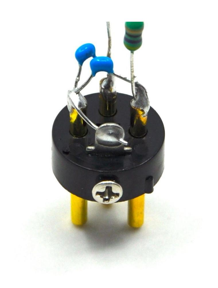
What must be added is that the microphone can function even without this filter. So there is nothing stopping you from trying the microphone without it. In this case, just connect pin 1 of the XLR connector to the GND pad on the board, pin 2 to the XLR 2 pad on the board and pin 3 to the XLR 3 pad on the board using a cable. If you have a problem with signal interference, you can finish the filter later.
