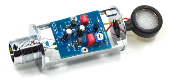
Put the head basket on the microphone and you can proceed to the first test of the microphone. Connect the microphone via cable to the preamp and activate phantom power.
