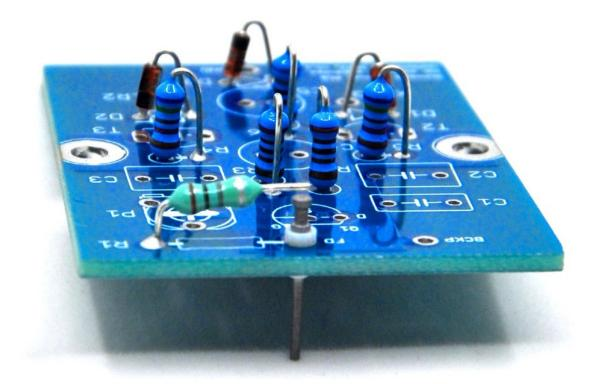
Continue by installing the FET transistor. I chose the original BC264, whose GATE leg is on its edge. If you choose another FET, keep in mind that the GATE leg may be elsewhere. Always check this against the data sheet of the particular FET transistor. Note that the GATE leg is also soldered in the air to the teflon pin.
