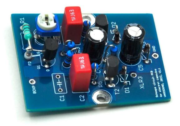
Clean the back of the board thoroughly with a brush and isopropyl alcohol to keep it perfectly clean and free of soldering debris.
