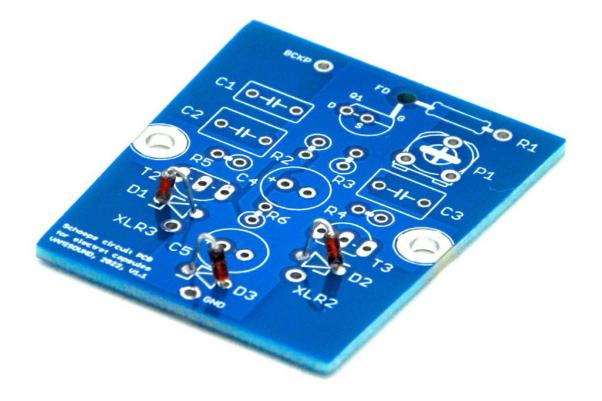
Continue by soldering resistors as in the picture. R2 and R3 form a matched pair, the same for R4 and R5.
