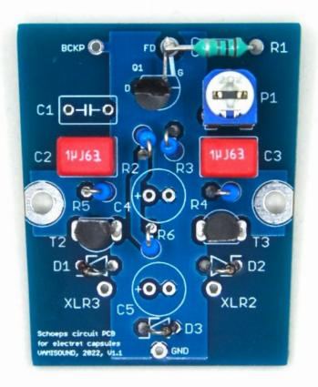
Two electrolytic capacitors remain to be installed.
